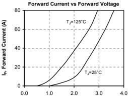
V<sub>F</sub>, Anode to Cathode Voltage (V)
