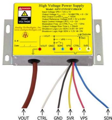
Figure 2. The Connecting Lead Wires of AHV12VN1KV1MAW
