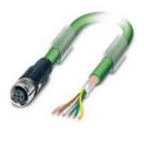
Bus system cable, INTERBUS (16 Mbps), 5-position halogen-free, shielded, free cable end, on Socket straight M12, coding: B SPEEDCON, cable length: 2 m
