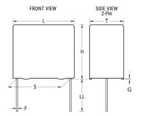
**General Information** Series PFR/F411 Dielectric Film/Foil Polypropylene Style Radial Features Pulse RoHS Yes Lead Wire Leads AEC-Q200 No Component 0.374 g Weight An Operating Temperature Up To +105C Is Allowed Under Certain Conditions. Please Consult Miscellaneous KEMET For Details.
