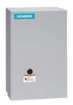
Electrically held lighting contactor, Contactor amp rating 30A, 0 N.C. / 12 N.O. Poles, 347VAC 60HZ coil, Non-combination type, (no disconnect device), Enclosure NEMA type 1, Indoor general purpose use
