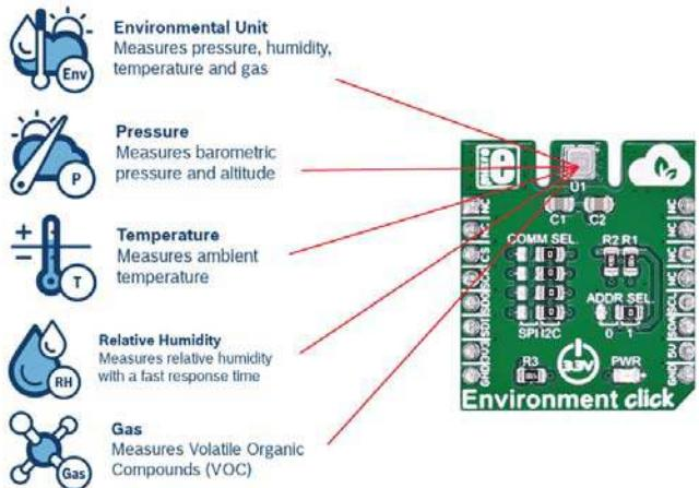
The **humidity sensor** provides an extremely fast response time for fast context awareness applications and high overall accuracy over a wide temperature range. The **pressure sensor** is an absolute barometric pressure sensor with extremely high accuracy and resolution.
