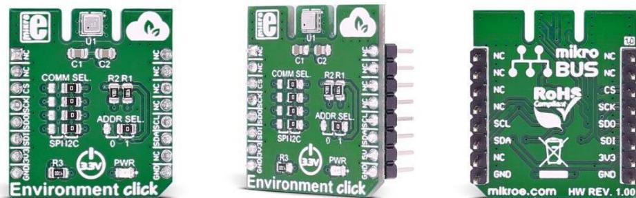
**Environment click** measures temperature, relative humidity, pressure and VOC (Volatile Organic compounds gases). The click carries the BME680 environmental sensor from Bosch. Environment click is designed to run on a 3.3V power supply. It communicates with the target microcontroller over SPI or I2C interface.
