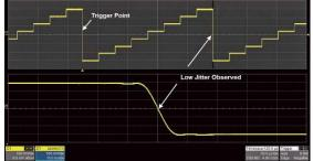
The Teledyne Test Tools T3AFG200, T3AFG350 and T3AFG500, with its low jitter design, can generate waveforms with exceptional edge stability. With better jitter performance comes better edge stability, and higher confidence in your circuit design.
