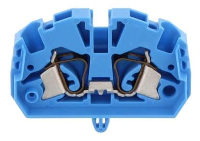
Feed-through terminal for direct mount, Tension-spring connection, Mounting type: Mounting surface, Rated cross-section: 2.5 mm<sup>2</sup>, Width: 5.1 mm, Colour: Blue
