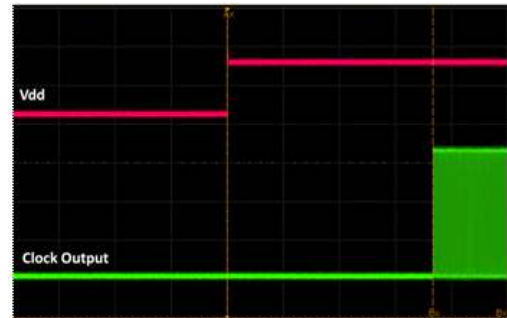
Figure 16. Startup Waveform vs. Vdd
