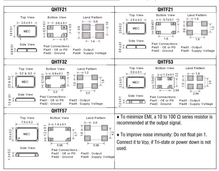
**Output OE Function on pad 1** Note: Do not leave this pad floating. If "no-connection" is desired, please contact Mercury.
