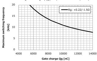
Ta:- $40\sim+85$ °C / VIN = 13.5 $\sim$ 18V Ta:- $40\sim+75$ °C / VIN = 18 $\sim$ 26.4V
