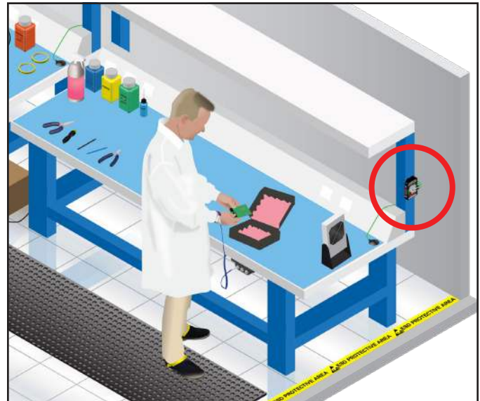
Figure 3. Installing the Common Point Ground Monitor at the end of a row of workbenches
