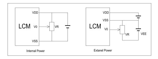
$V_{DD^{\sim}}V_0$ : LCD Driving voltage
