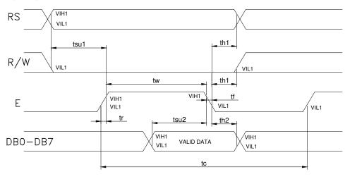
Read cycle (Ta=25 $^{\circ}$ C, VDD=5.0V)
