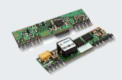
Advanced Energy's Artesyn SIL10E series of non-isolated DC-DC converters comprises eight fixed output models covering voltages from 0.8 to 3.3 Vdc and one wide output trim model that can adjusted over the range 0.8 to 3.63 Vdc. All models can deliver up to 10 amps output current. The 3.3 V fixed output and trimmable models accept a 4.5 to 5.5 Vdc input, while all other fixed output models accept a 3 to 5.5 Vdc input.
