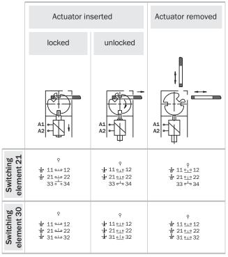
→ Positive action N/C locking monitoring contact
