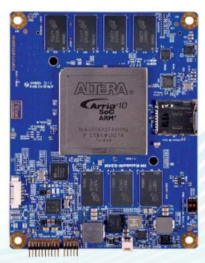
iWave's Arria 10 SoC System on Module is based on the Arria 10 SX family device with F34 package. The module is equipped with 32-bit DDR4 PS memory support for HIVith ECC and 64-bit DDR4 support for FPGA. All d the IOs and high speeransceiver blocks will be available on the SOM board to board connectrs.
