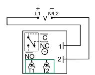
V = Voltage C = Common NO = Normally Open NC = Normally Closed T1 = OFF Time T2 = ON Time
