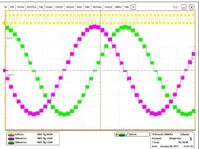
Figure 29. 1/8 Microstepping With Mixed30-Mixed30 Decay
