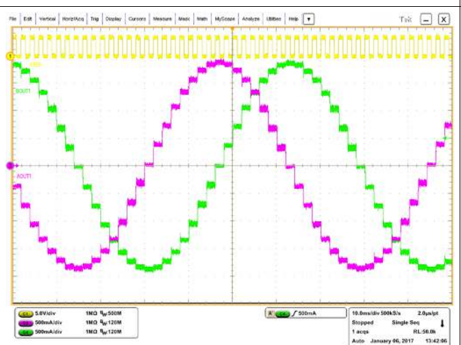
Figure 29. 1/8 Microstepping With Mixed30-Mixed30 Decay
