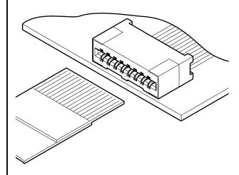
The FMS series connectors are designed for surface mounting (SMT) and to meet the demand for high-density packaging. They are miniature connectors with a height of only 2.8 mm, and can be supplied packaged in embossed tape to facilitate automatic mounting.
