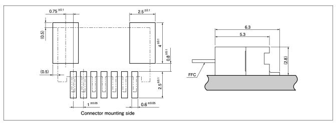
Note: 1. Tolerance for the PCB pattern pitch shall be  $\pm\,0.05$  and shall not accumulate.
