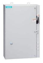
Reversing motor starter, Size 0, Three phase full voltage, Solid-state overload relay, OLR amp range 5.5-22A, 110V 50Hz / 120V 60Hz coil, Combination type, 25A circuit breaker, Enclosure NEMA type 4/12, Water/dust tight for outdoors
