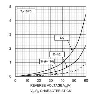
REVERSE POWER DISSIPATION:P<sub>R</sub>(W)
