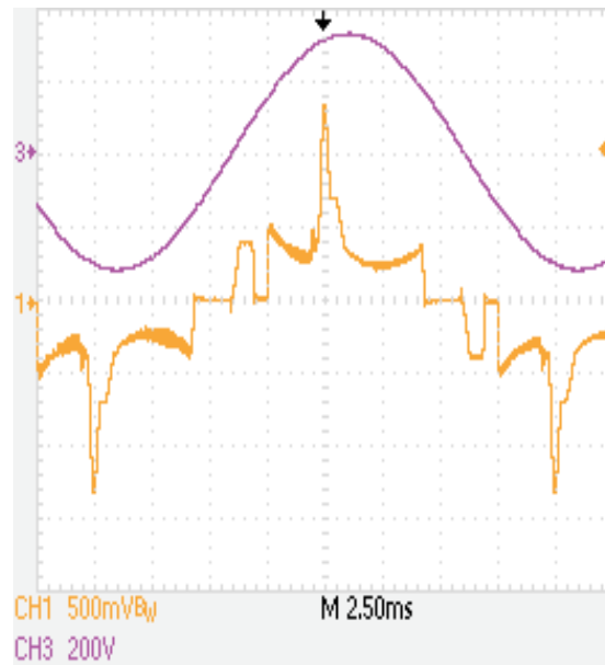
Figure 11. Input AC Voltage and Current, Full Load, no Dimmer, CH1 = I_{IN} , CH3 = V_{IN} , scale = 1 Amp/V
