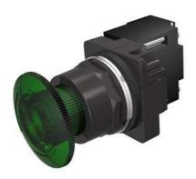
30mm BlackMax, Epoxy Coated Corrosion Resistant Metal Operator, Round Illuminated Twist-to-Release Transformer type, 120V AC Incandescent Lamp Mushroom Head Cap Small 1.79" (45 mm) Plastic Cap, Green 2 Position Maintained, Twist-to-Release UL Listed, CSA Certified NEMA 1,3,3R,4,4X,12,13 & Automotive Standards
