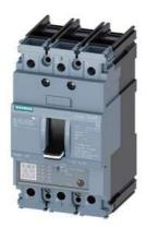
circuit breaker 3VA5 UL frame 125 3-pole, starter protection TM120M, AM, In=15A without overload protection short-circuit protection Ii=3...7 x In cable connection on both sides
