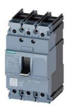
circuit breaker 3VA5 UL frame 125 breaking capacity class M 35kA @ 480 V 3-pole, line protection TM210, FTFM, In=50A overload protection Ir=50A fixed short-circuit protection Ii=10 x In UL489 SB (naval), 50 deg. cel. cable connection on both sides
