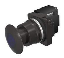
30mm BlackMax, Epoxy Coated Corrosion Resistant Complete Metal Unit Illuminated Push-Pull Operator Transformer type, 480V AC LED Lamp Mushroom Head Cap Small 1 3/4" (44.5 mm) Metal, Black with Blue Lens 3 Position Pull-Momentary/Push-Maintained UL Listed, CSA Certified NEMA 1,3,3R,4,4X,12,13 & Automotive Standards
