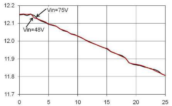
Figure 10. Typical Output Voltage Regulation vs. Output Current for the -P Option.
