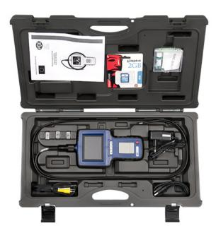
PCE-VE 340N is an industrial borescope, inspection camera or industrial endoscope for the non-destructive inspection (NDI) of engines, machines and more. This industrial borescope is an ideal tool for diagnosing issues in hard-to-reach places. The waterproof camera head features 4 LED lights with automatic illumination. In addition, digital image magnification or zoom of up to 2 times is available.
