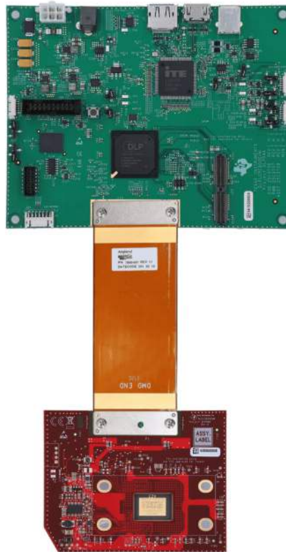
Figure 5-9. Assembled DLPLC900EVM with DLPLCR65EVM
