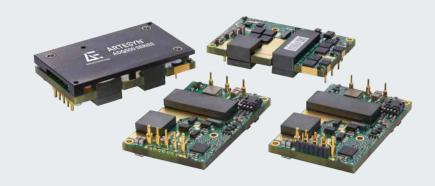
ADQ500 series quarter-brick isolated DC-DC converters produce a single fully regulated 12 V output. Rated at 500 watts, these converters can deliver up to 42 amps output current and have no minimum load requirement. They have an input voltage range of 36 to 75 V and are primarily designed for use with standard 48 V supplies in computing and server applications, as well as regulated 48V supplies in communications equipment.
