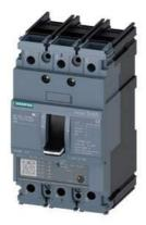
circuit breaker 3VA5 UL frame 125 3-pole, starter protection TM120M, AM, In=3A without overload protection short-circuit protection Ii=3...7 x In nut keeper kit on both sides
