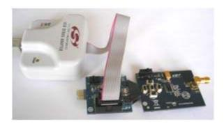
This setup is suitable for downloading, running, and debugging the program in RAM. This board has a PCB antenna and battery, so after downloading the program and starting the execution by disconnecting in the IDE, the board can be physically disconnected from the programming interface and tested in mobile form. A switch is provided on the board to connect/disconnect the battery.
