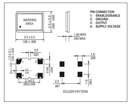
NOTE: A capacitor of 0.01  $\mu F$  between Vcc and Ground is recommended
