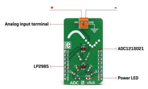
ADC converters in general, use a range of different mechanisms to convert the voltage on their input terminals. The ADC121S021 AD converter uses the SAR, or the successive approximation method for the conversion, which consists of comparing the input voltage with a series of internally generated voltage values. At each step in this process, the approximation is stored in a successive approximation register. The comparing steps are continued until the desired resolution is reached.
