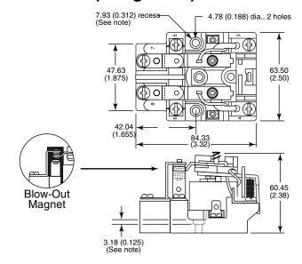
Note: Recess for screw mounting on units with 300-600 VAC coils
