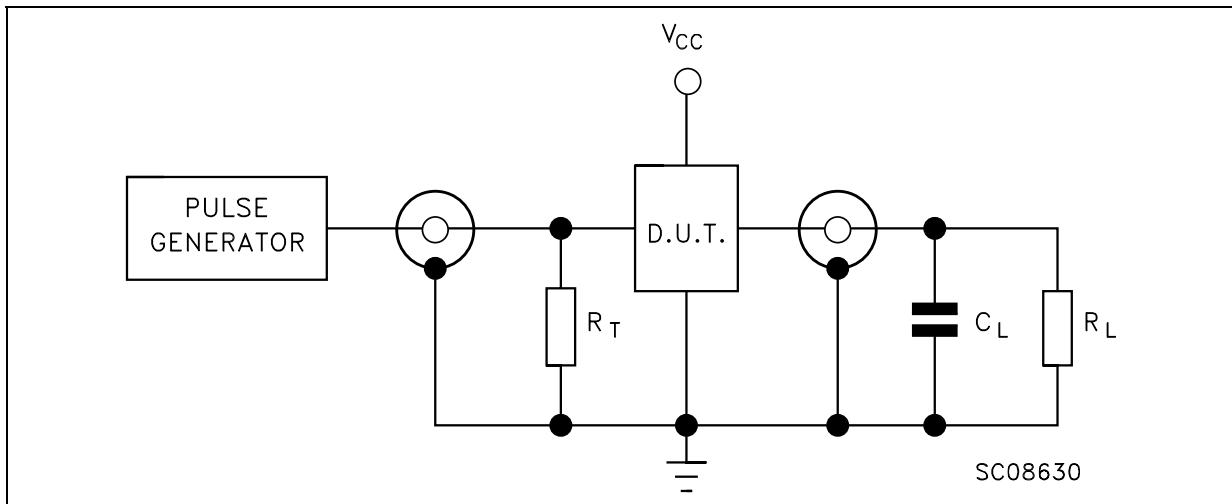
**TEST CIRCUIT AND WAVEFORM SYMBOL VALUE**
