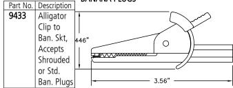
**Construction:** Insulator is molded nylon. Alligator jaws and banana socket are formed steel nickel plated. IEC 1010 rating: 1000 Volts Cat III, 30 amps. **Colors**: Black, red, green, blue, yellow, white.
