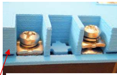
Connexions de commande M4 M4 control connections
