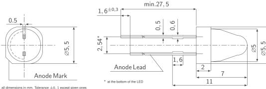
all dimensions in mm. Tolerance  $\pm 0$ , 1 except given of
