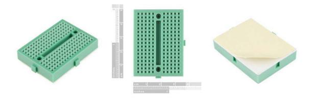
**Description:** This green Mini Breadboard is a great way to prototype your small projects! With 170 tie points there's just enough room to build and test simple circuits; They're also great for breaking out DIP package ICs to jumper wires! If you run out of room, no worries, these mini breadboards can be snapped together to form larger stretches of board. It has a peel and stick adhesive backing as well as two mounting holes for M2 screws so you can anchor it down.
