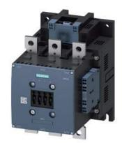
power contactor, AC-3e/AC-3 225 A, 110 kW / 400 V AC (50-60 Hz) / DC Uc: 200-277 V PLC input 24 V DC 3-pole, auxiliary contacts 2 NO + 2 NC drive: electronic main circuit: busbar control and auxiliary circuit: spring-loaded terminal
