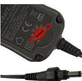
(3) Insert correct plug with GND outside
