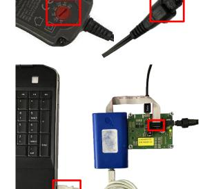
3) Connect USB-cable to Interface-Board and PC
