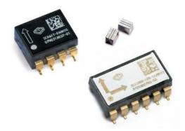
The SCA Demo Kits are designed for VTI Technologies (MEMS) accelerometers. They can be used for research and evaluation purposes in different applications where physical movement will be converted to an electrical signal.
