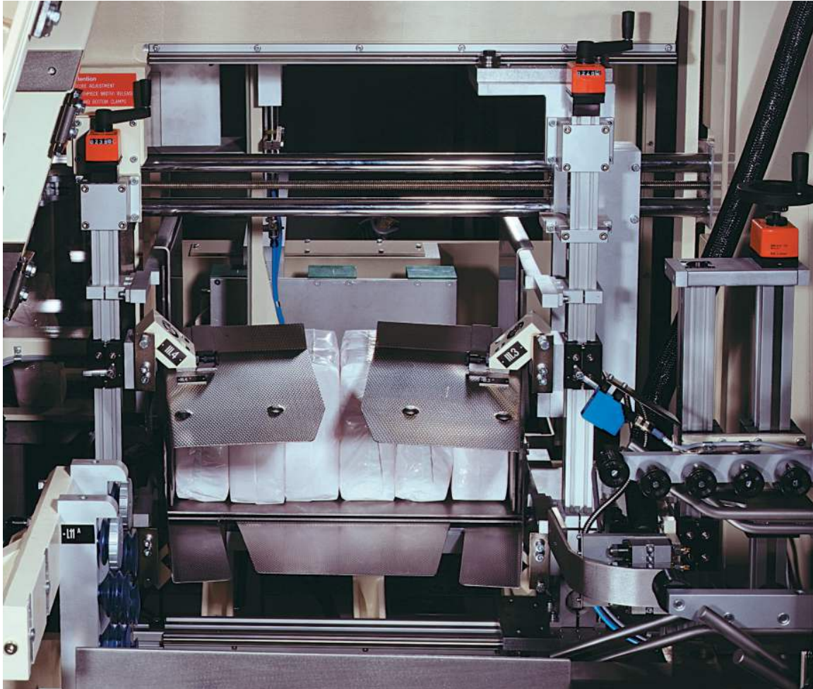
Simple fixation of linear units (for format adjustment) on a packaging machine.
