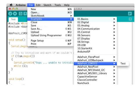
Open the special Adafruit version of the Arduino IDE and naviate to File-->Examples-->Adafruit\_LSM303-->Test to open the accelerometer test sketch. For more information on programming the Flora, check out the Getting Started with FLORA () guide.
