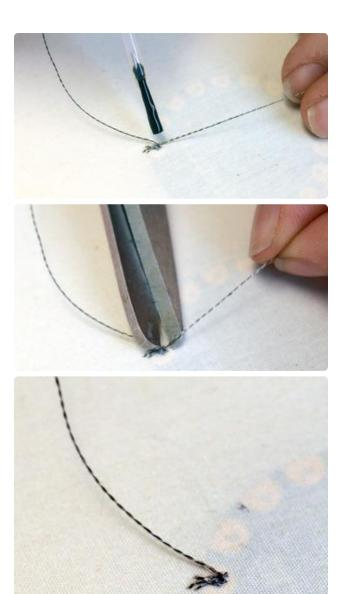
Dab a little Fray Check or clear nail polish on the knot while holding it tight. This will prevent the knot from coming undone and creating unwanted shorts in your circuit. Trim the tail very close to the knot.
