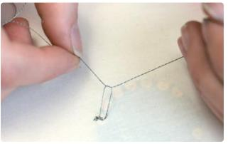
Stitch a few times around the GND pad and end on the back side of the fabric. Tie the tail and the working thread into a square knot, tight against the fabric.
