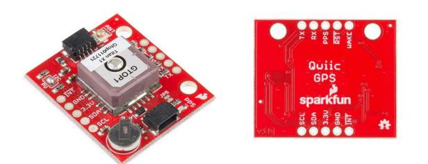
The SparkFun XA1110 GPS Breakout is a small I<sup>2</sup>C-supported module built for easy hookup, thanks to our Qwiic Connect System. Equipped with the XA1110 GPS module from GTOP, this board utilizes the MediaTek MT3333 chipset, loaded with specialized SparkFun firmware that enables both I<sup>2</sup>C and serial ports simultaneously. Using I<sup>2</sup>C means you won't have to tie up your serial port with GPS, leaving it open to other possibilities.
