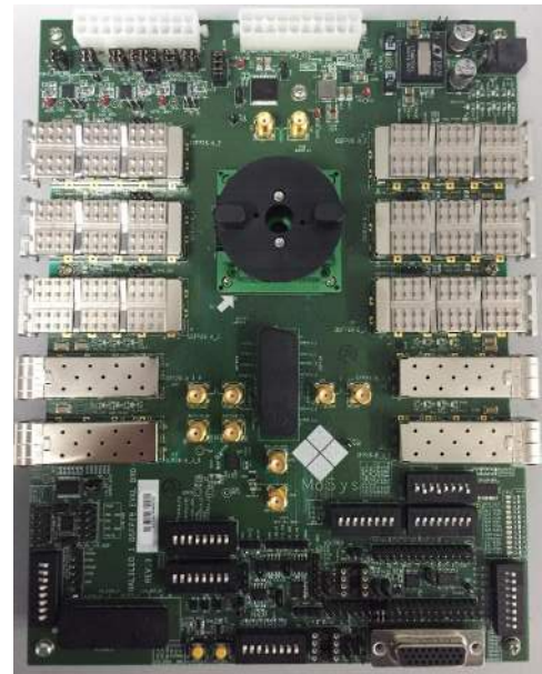
17x17mm QSFP28 Evaluation Board and reference
