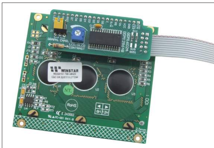
Figure 5: Serial LCD/GLCD Adapter additional board with a 128x64 GLCD (jumper J1 in GRAPH position)
