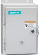
Non-reversing motor starter, Size 0, Three phase full voltage, Solid-state overload relay, OLRelay amp range 0.25-1a, 220 240/440 480VAC 60HZ coil, Non-combination type, Enclosure type 12, Dust/drip proof for indoors, Extra-wide enclosure
