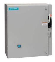
Non-reversing motor starter Size 3 Three phase full voltage Solid-state overload relay OLRelay amp range 25-100A 380-440/440-480V 50/60HZ coil Combination type 125Amp circuit breaker Enclosure NEMA type 1 Indoor general purpose use Standard width enclosure
